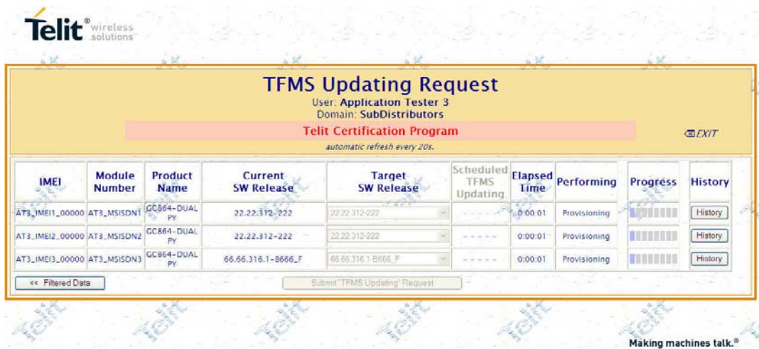
Fig.15 Performing the dummy update, provisioning phase in progress
